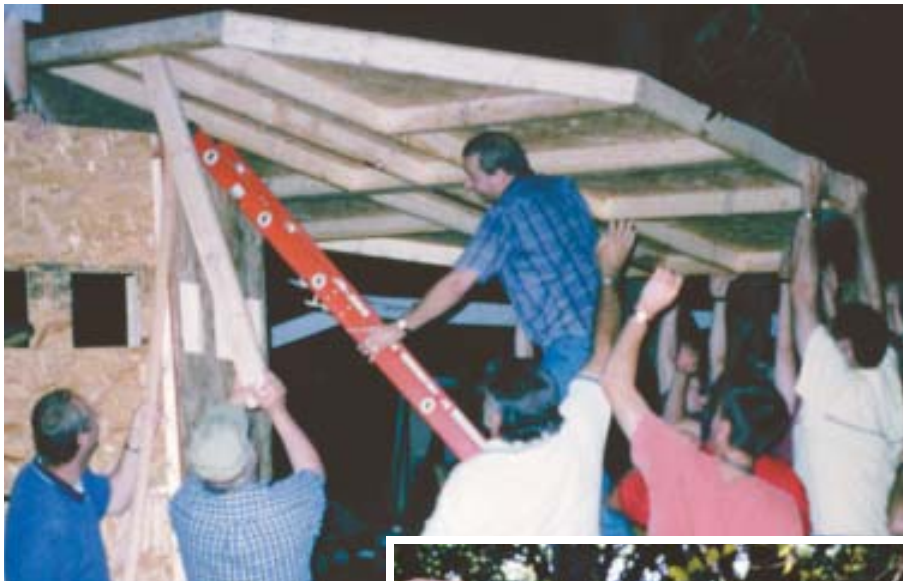
Figure 4. The author and his colleagues tested 21 different combinations of building papers and claddings on this eight-sided structure (above). Measuring the added water (right) provided a basis for comparing results across wall systems. The blower door apparatus (far right) turned out not to matter, because leaks were apparent without any air pressure difference.
