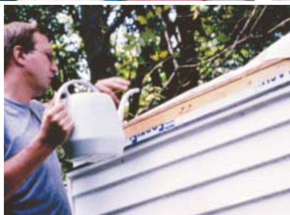
Figure 4. The author and his colleagues tested 21 different combinations of building papers and claddings on this eight-sided structure (above). Measuring the added water (right) provided a basis for comparing results across wall systems. The blower door apparatus (far right) turned out not to matter, because leaks were apparent without any air pressure difference.
