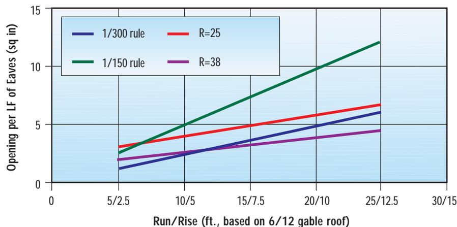
This graph shows required vent area as calculated by the 1/300 and 1/150 rules compared with CRREL calculations based on building size, roof slope, and insulation levels. In most cases, the 1/150 rule provides more than adequate venting area, even at lower insulation levels; the 1/300 rule also works well for well-insulated attics. However, for small buildings, such as those depicted at the extreme left end of the chart, these rules of thumb may fall short.
