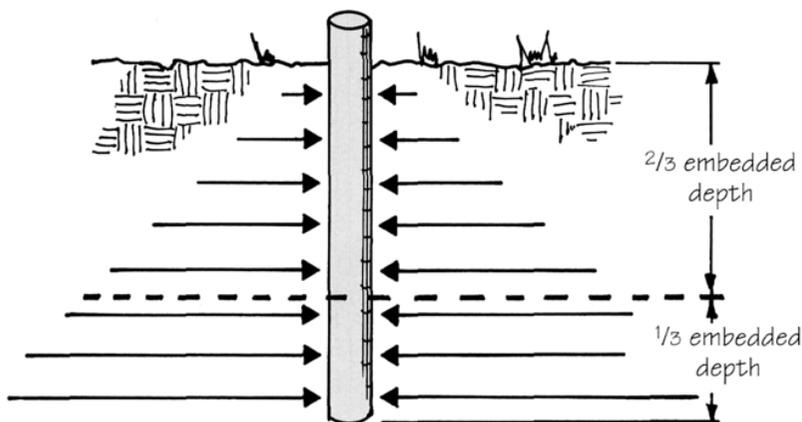
**Figure 1.** The pressure of the earth against an embedded post increases as the post goes deeper. According to the Coulomb theory, the pressure against the bottom third of the post equals the pressure against the top two-thirds.
