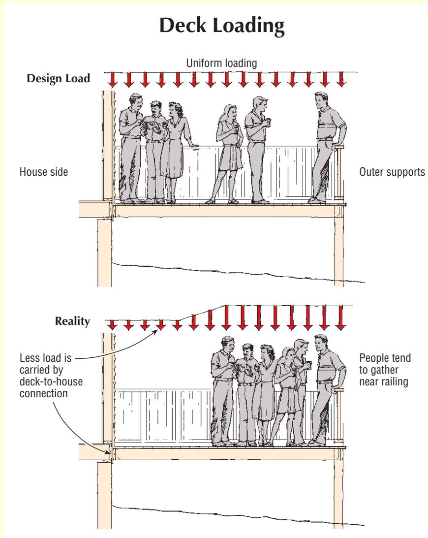
Decks are designed for uniform loading (top). In reality, people tend to gather near the railings rather than next to the house, taking some of the load off the ledger (above).
