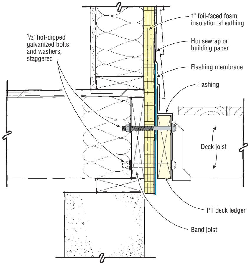
The authors used available *NDS* methods to create a fastener schedule that accounts for a drainage space behind a ledger attached over 1/2-inch sheathing (above left). Unfortunately, the sheathing provides no structural support to the bolt, resulting, from a design standpoint, in a 1-inch-wide gap between the ledger and the band. Thus, the same bolting schedule would apply to a ledger installed over 1-inch nonstructural insulating sheathing (above).
