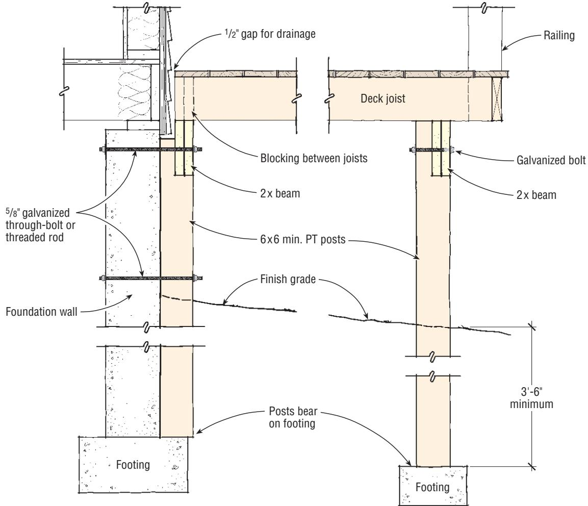
The authors strongly recommend avoiding mechanical shear connections altogether and, instead, supporting residential decks with PT posts, as shown here. Use .60-retention pressure-treated lumber for greatest durability.
