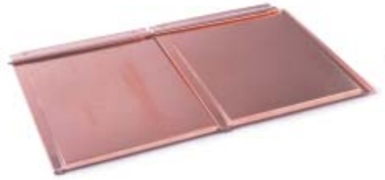
Figure 14. Copper, used for centuries to make long-lasting standing-seam panels, has more recently lent its longevity and beautiful coloration to shingle-style panels like these from Zappone. The locking hems on these shingles, also found on steel and aluminum styles, give them unsurpassed wind resistance.
