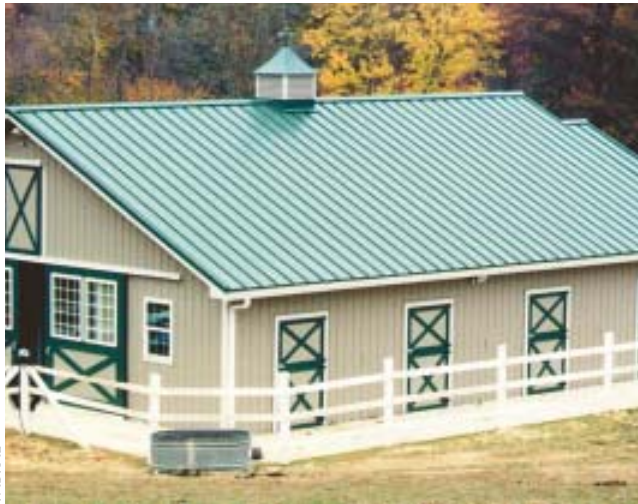
Figure 1. Exposed-fastener metal roofing has long been used for barns and industrial buildings because it's inexpensive, installs quickly, and lasts 30 or 40 years. It also makes a great residential roof in areas with a rural character, especially in hot or snowy regions.
